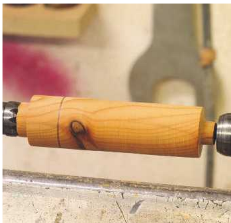
▲ Pic.28 The small arms are mounted between centres and roughed round to about 20mm. Turn the spigot on one end and take the waste down at the headstock end
